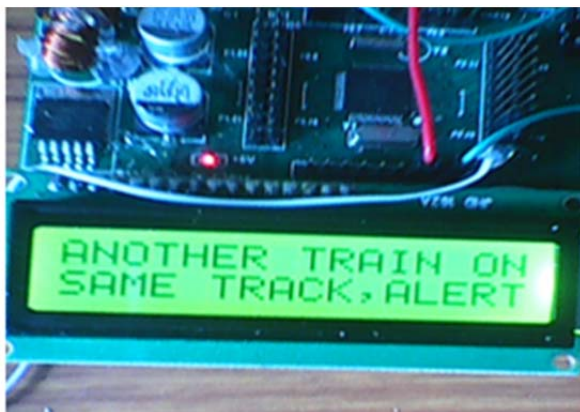
FIG-6: DISPLAY OF ALERT MESSAGE WHEN TWO TRAINS ARE IN SAME TRACK
